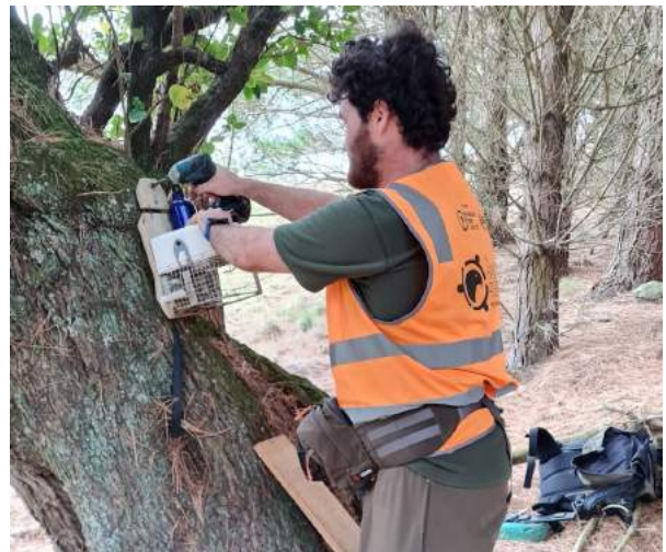
Installing the first AT220 automated trap.
